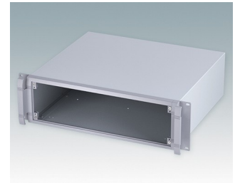
M5619335 UNIMET 19" 3HEx380mm Aluminium Lichtgrau/fenstergrau RAL 7035/7040 132.5x482.6x380mm
